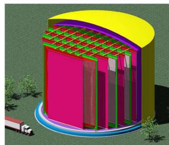
The ultimate goal of LARTPC R&D: a **50 kiloton chamber**, pictured here with an 18-wheeler for scale.
