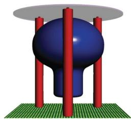
Current design for PMT module in MicroBooNE. A plate (in gray) coated with a wavelength shifter is fastened in front of PMT to shift UV light to blue light.
