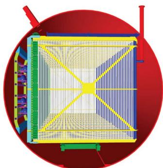
PMTs in MicroBooNE can only be placed in the zero field side of the chamber, behind the wire planes. This lack of coverage limits the ability to detect light events in the detector.
