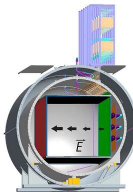
Side views of **MicroBooNE**, a LARTPC that will soon be under construction at Fermilab. It will have a fiducial volume of ~70 tons.
